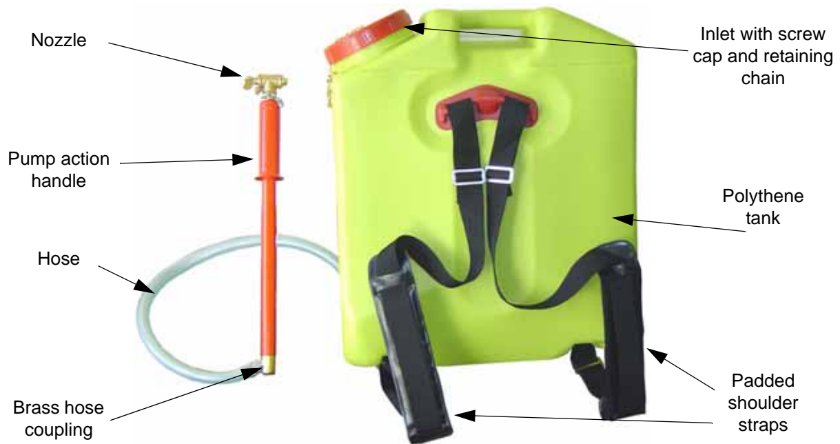
Figure 3 Hard knapsack main components
